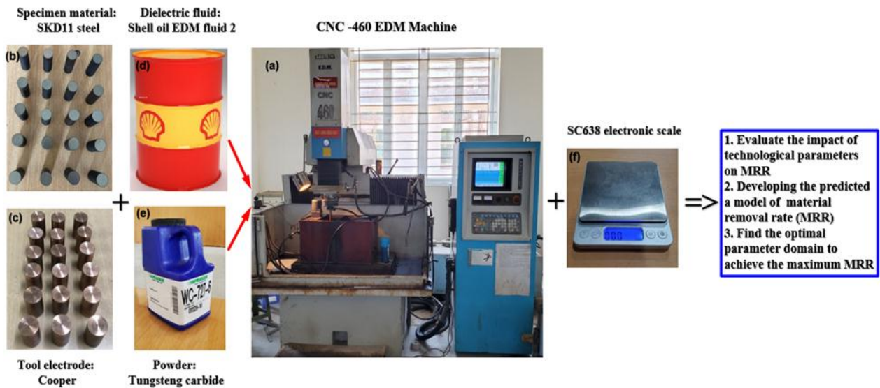
Figure 1: (a) EDM CNC-460 machine, (b) the specimen material, (c) the tool electrode material, (d) the dielectric liquid, (e) the powder, and (f) electronic scale
