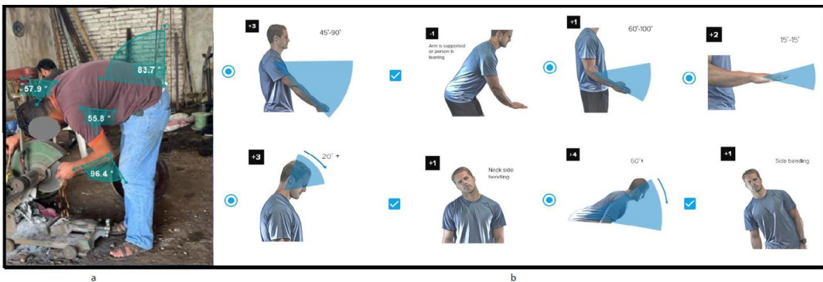
Figure 8. (a) An operator performing a grinding task (b) RULA assessment - grinding task
