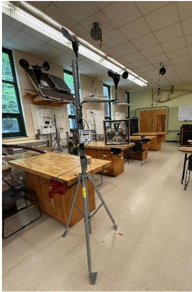
Figure 8: Lab-scale Met tower and sensor assembly
