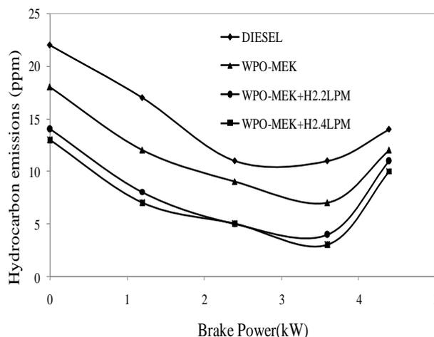
Fig. 6 Variation of hydrocarbon emission with brake power
