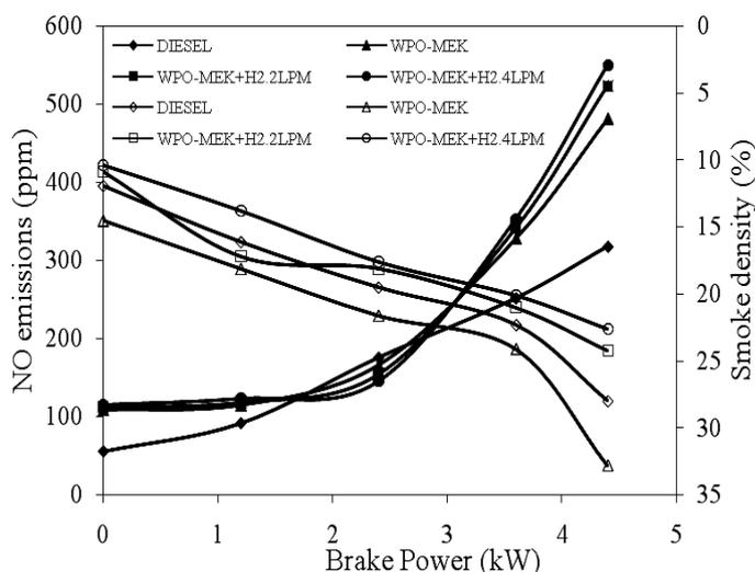
Fig. 8 Variation of the NO and smoke emissions with brake power
