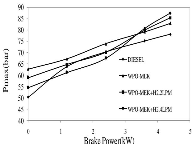
Fig. 4 Variation of the cylinder peak pressure with brake power
