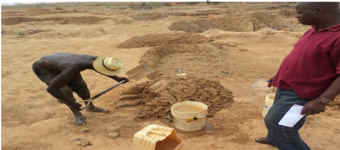
Plate 1. Illustrate mixing procedure for brick making
