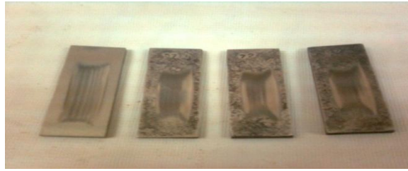
Figure :4 Specimens after wear test of AR and HT at Different temperature at 6 kg load
