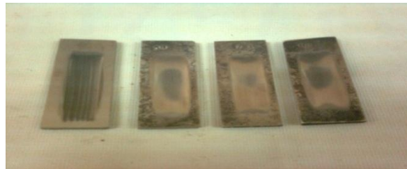
Figure :5 Specimens after wear test of AR and HT at Different temperature at 13 kg load
