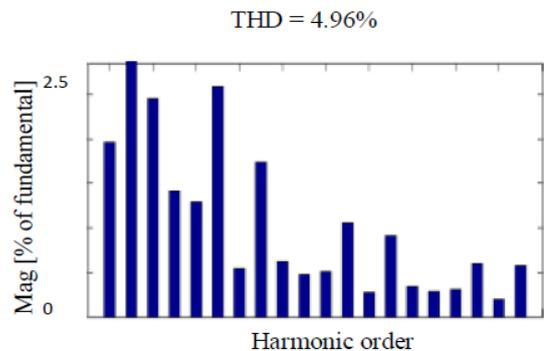
Figure 10. Spectrum analysis of supply current-after compensation using PPF
