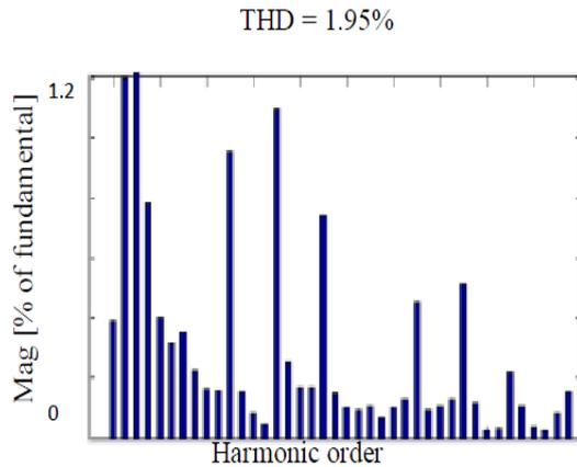
Figure 16. Spectrum analysis of supply current- after compensation using SAPF and PPF
