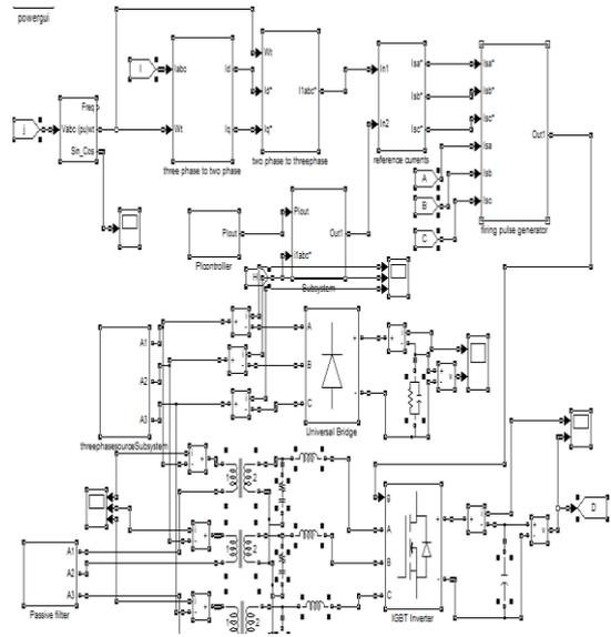
Figure 14. Simulation diagram with APF and PPF
