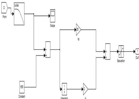
Figure 4 PI-controller using indirect current control technique.
