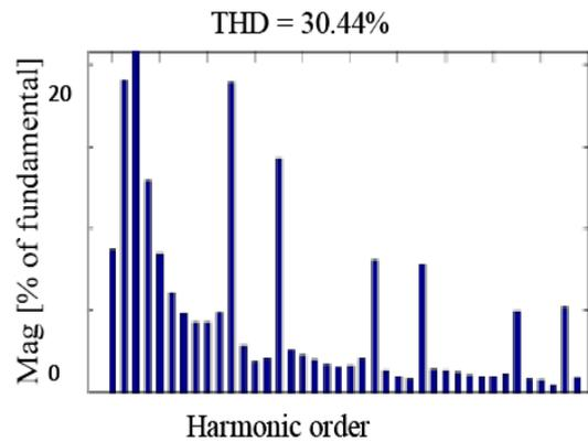
Figure 8. Spectrum analysis of supply current-before compensation.
