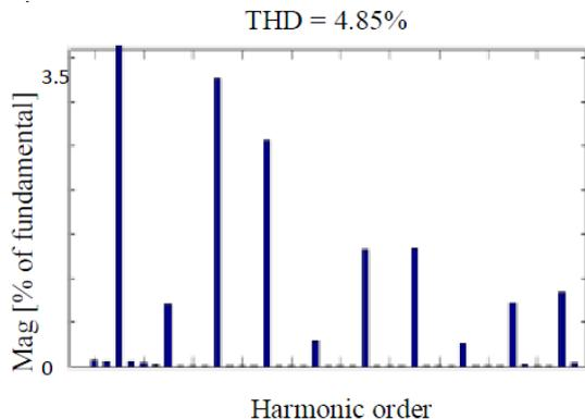
Figure 13. Spectrum analysis of supply current after compensation using APF.
