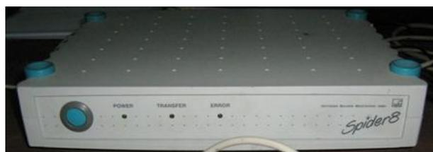
Fig. 6. The data acquisition system SPIDER 8
