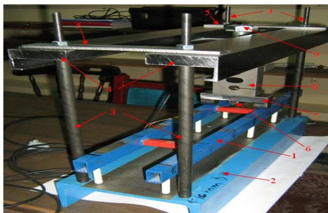
Fig. 2. The device used to bend parts of the studied metallic structure. General view
