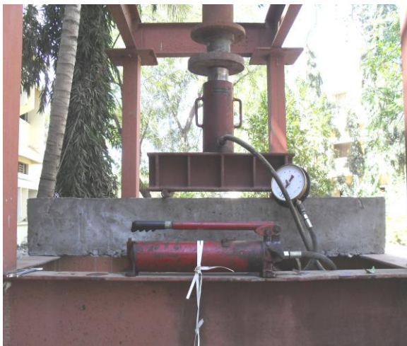
Plate 1 Loading Frame Arrangement & Application of Chicken Mesh on Beam Surfaces
