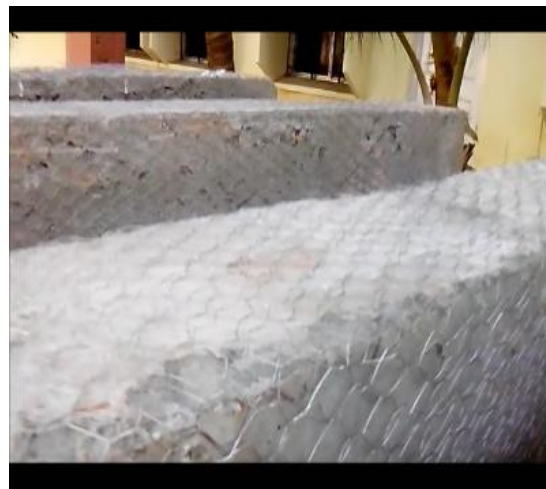
Plate 1 Loading Frame Arrangement & Application of Chicken Mesh on Beam Surfaces
