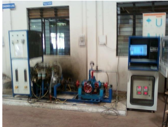
Fig.1.Experimental Set Up With Hydraulic Dynamometer.
