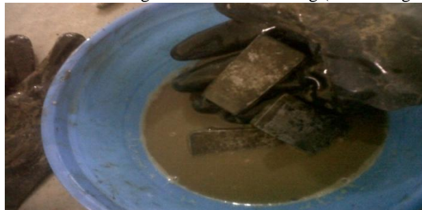
Fig. 3.6 Washing the coupons
