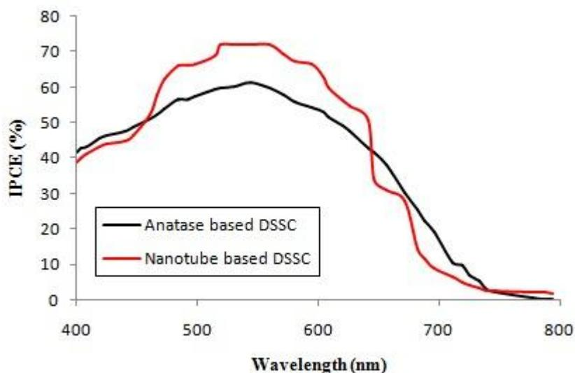
Figure 4. IPCE curves for nanocrystalline and nanotube based DSSCs
