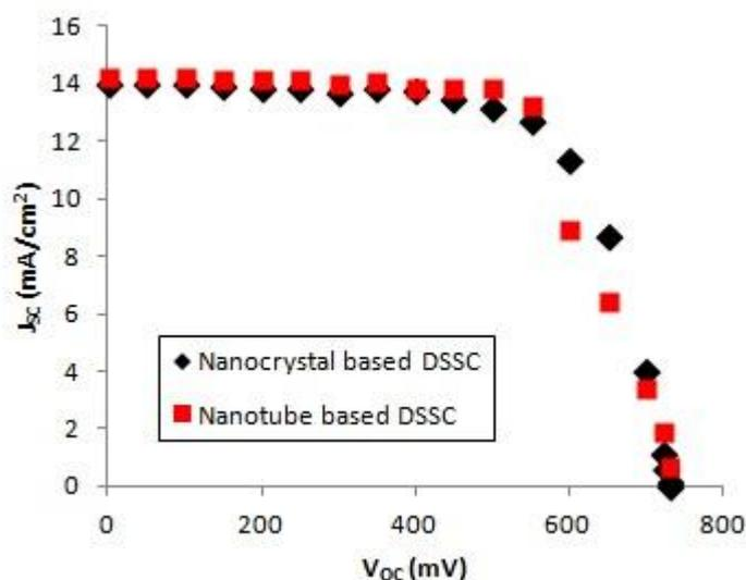
Figure 3. JV characteristics of fabricated DSSCs
