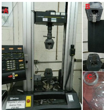
Figure 4. a) Set up used for the tensile tests, b) sample fixing in the clamps, c) recycled PET fiber specimen.
