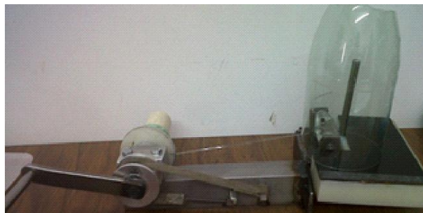
Figure 2. Device used to obtain the PET fibers.
