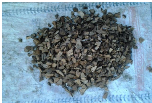
Figure 3: Coconut shell as aggregates
