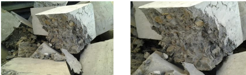
Figure 6: Coconut Shell Blended Concrete Cube Specimen after Test
