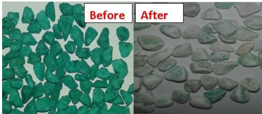
Figure 6: Images of dolomite particles before and after attrition
