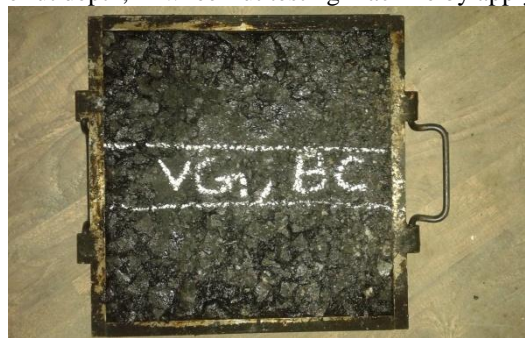
Figure4.4 Wheel Rut Sample Before Testing
