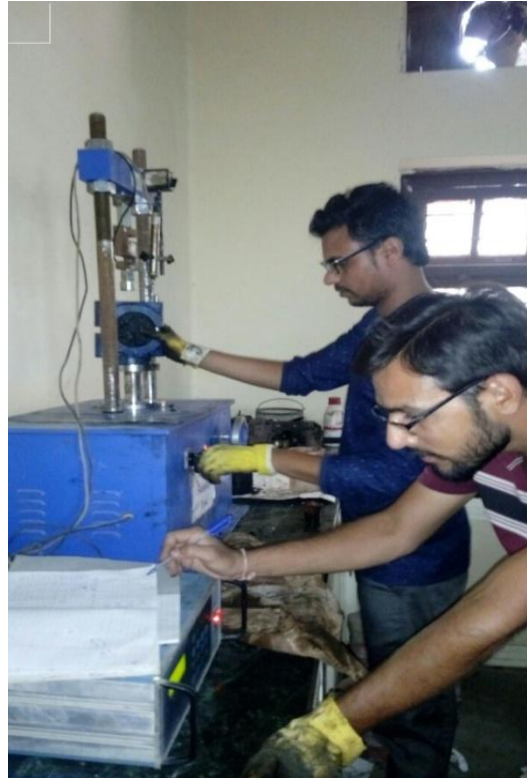
Figure4.3 Marshall Stability Testing
