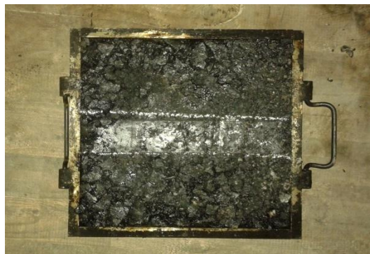
Figurte4.5 Wheel Rut Sample After Testing
