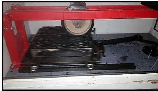
Figure 5.1 - Wheel rut testing machine with specimen
