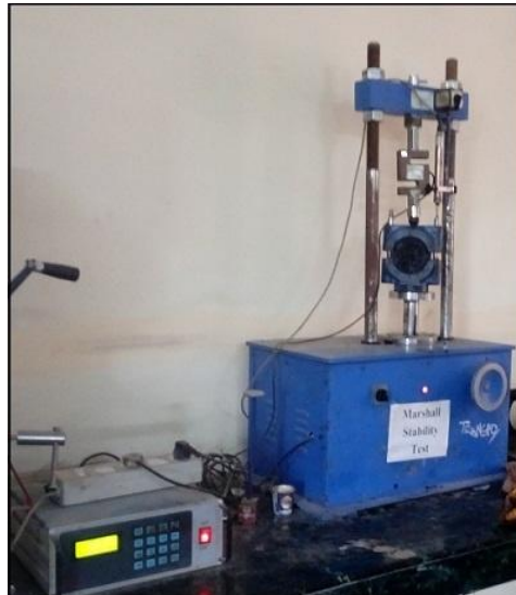
Figure 3.1- Marshall Stability Testing Machine
