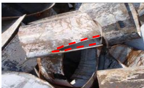
Figure 5. The piece of tube was found in borehole A2 (the red line shows the cut portion of this).
