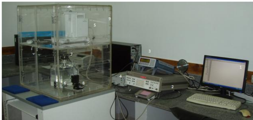
Fig. 2: A photograph of the primary RFB system at NIS of Egypt.
