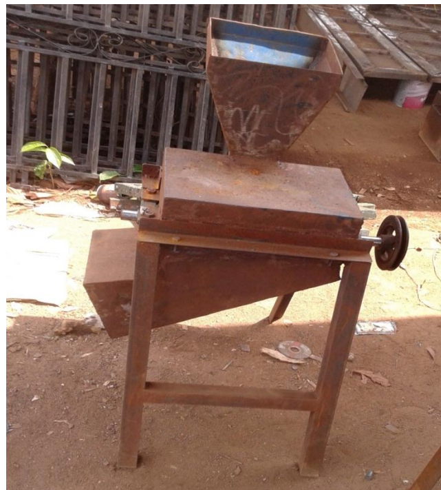
Figure 3: The Fabricated Crusher
