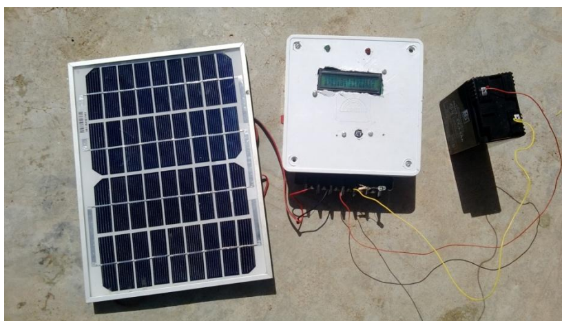
Figure.9 Pictorial Diagram of Complete Constructed Solar Charge Controller During Test.
