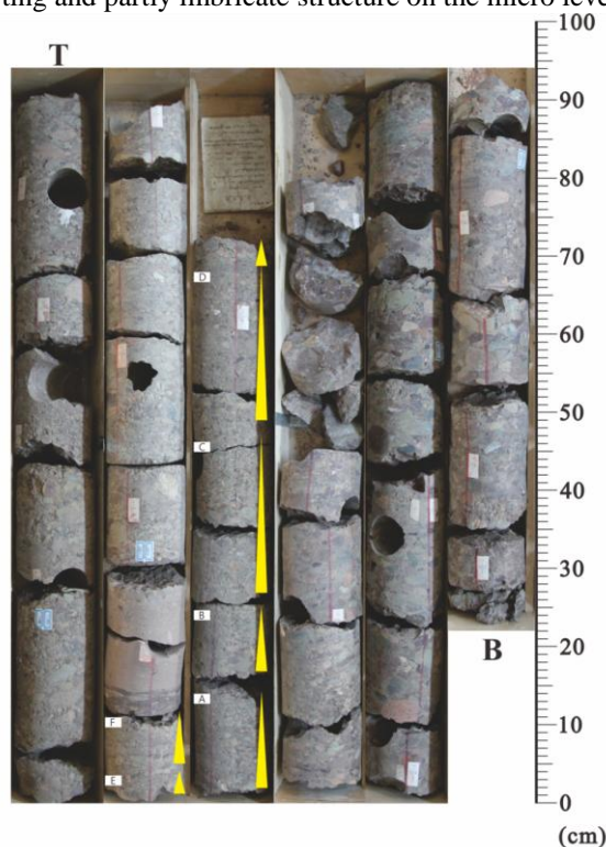
Fig. 5 M001 well core photographs (3486.00-3491.07m) showing multiple positive grain sequences.
