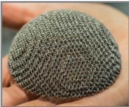
Fig.2.4. Components produced by EBM ( https://additivemanufacturingllc.com )
