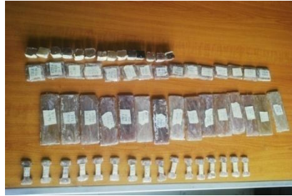
Fig. 5. Samples prepared with unsaturated polyester resin
