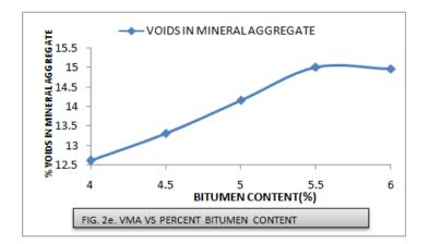
Optimum Bitumen Content =  $\frac{A+B+C}{3}$  (1)
