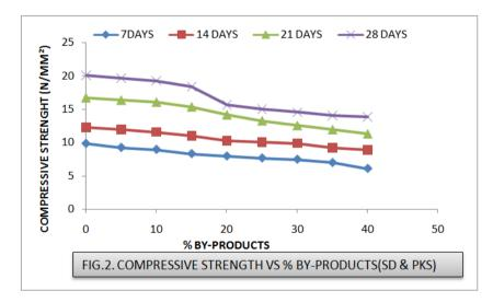
Although the compressive strength reduces as by product concentration increases, the compressive strength obtained to 15% by products addition meets the criterion for light weight concrete as they have mean compressive strength value above  $17N/mm^2$  (NRNCA, 2017). The reduction in compressive strength may be attributed to the smooth and nature of PKS, thereby making it difficult to bind well with cement upon hardening.
