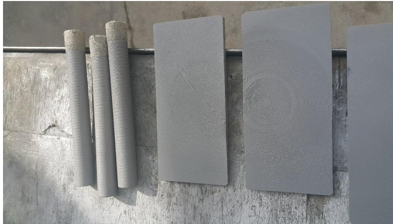
Fig. 1 Flat and cylindrical samples of plain carbon steel brass coated.
