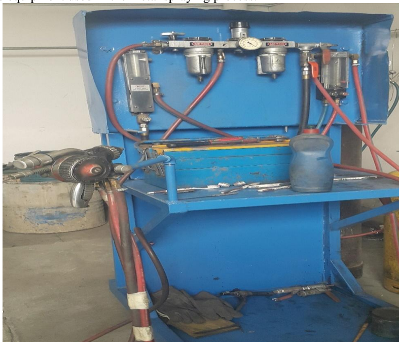
Figure 1: Equipment used in the process of brass metal spraying on plain carbon steel
