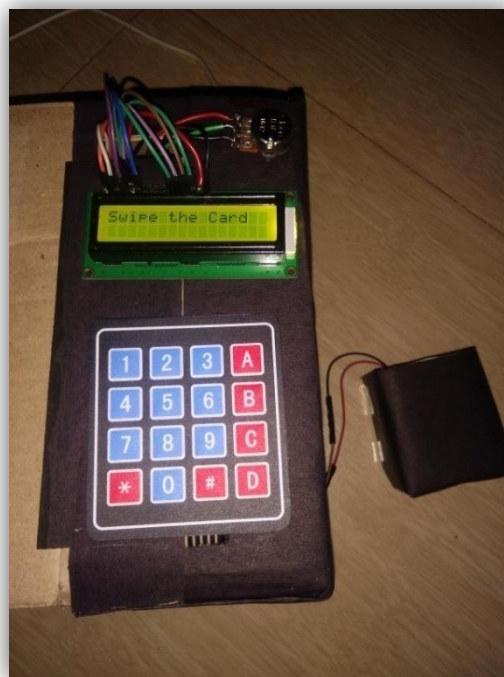
Fig 4. LCD DISPLAY PROMPT MESSAGE "SWIPE THE CARD".
