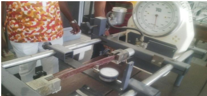
Plate 4: Bending test sample on fix support at both ends.
