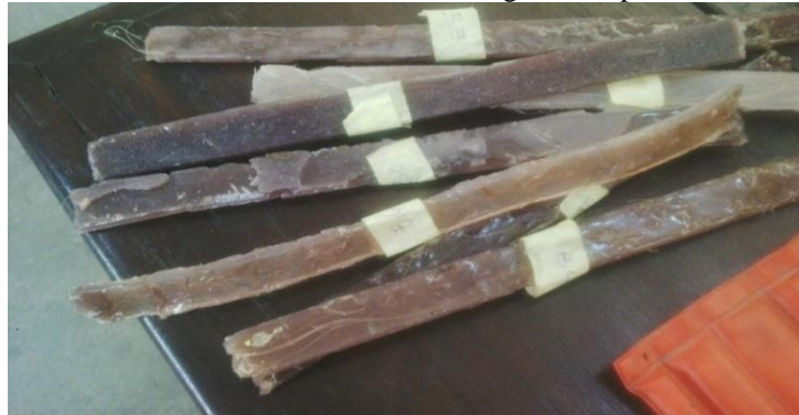
Plate 7: Samples after bend test
