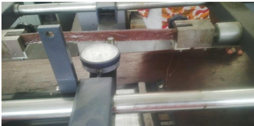
Plate 5: Bend test sample under induced force of 200N
