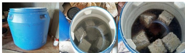
Figure 7 Cubes immersed in 5% H_2SO_4 solution for 60 days and after 60 days ready for acid attack test
