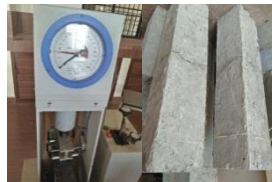
Figure 6 Flexural strength test setup and cracked beam
