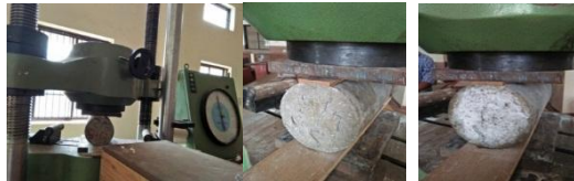
Figure 5 Split tensile strength test setup, initiation and propagation of cracks in cylinders
