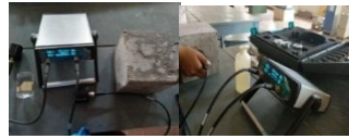
Figure 8 UPV test set up to measuring velocity
