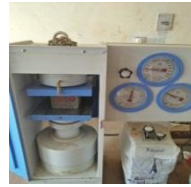
Figure 4 Compressive strength test setup
