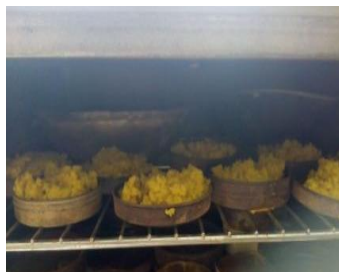
Plate 3: Oven drying of ARH
