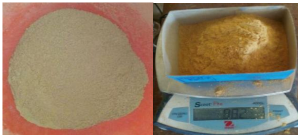
Plate 4: ARH after grinding and sieving
