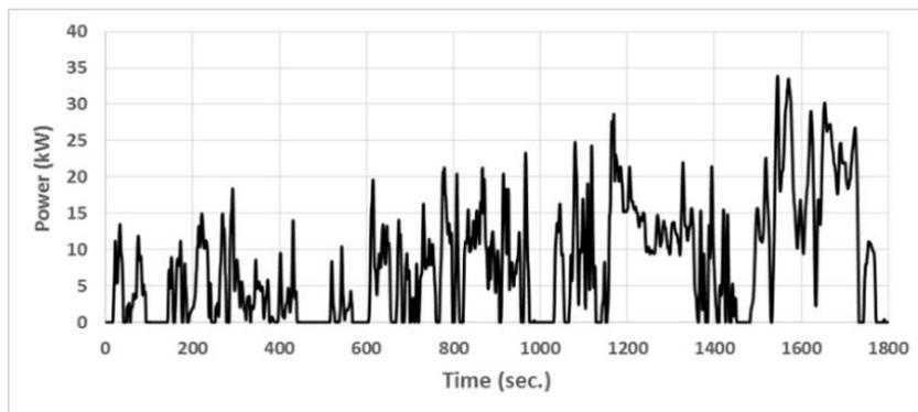
Figure7: Wheel Power during WLPT Cycle.
