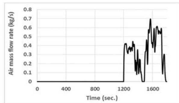
**Figure 12.** Cooling fan air flow rate with LQR
