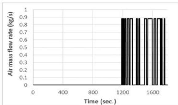
**Figure 11.** Cooling fan flow rate in conventional system
