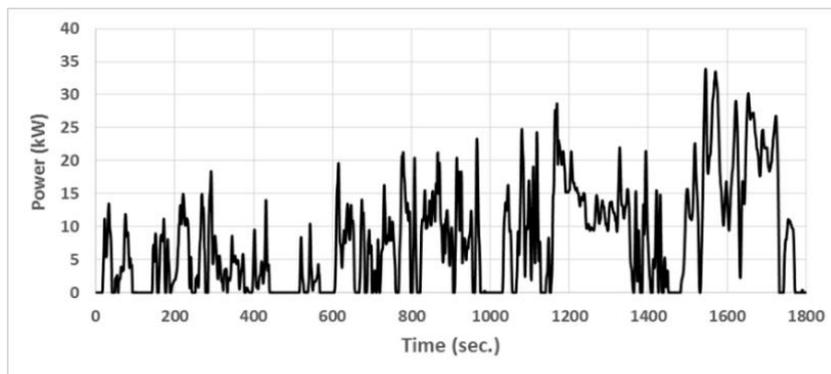
**Figure7:** Wheel Power during WLPT Cycle.
