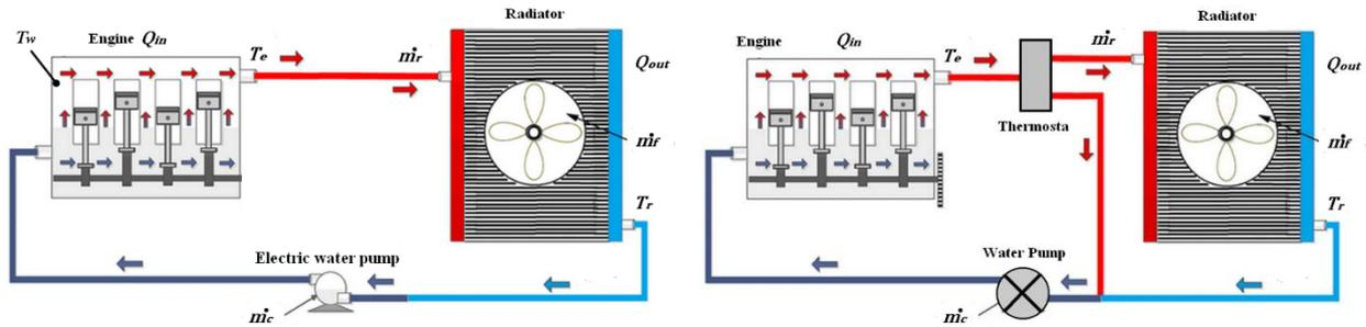
Figure 1a. Electrically controlled cooling system layout. Figure 1b. Conventional cooling system layout.
