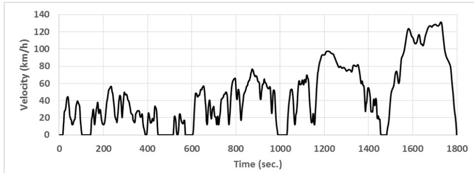
**Figure 6.** Vehicle Speed during WLTP Cycle.
