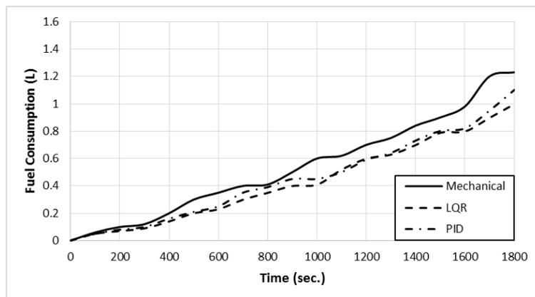
**Figure 14.** Engine fuel consumption during WLPT cycle for the three systems.
