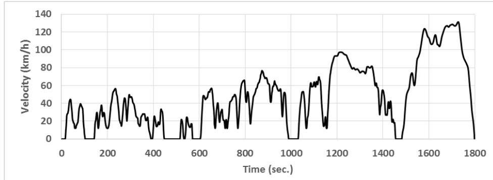
Figure 6. Vehicle Speed during WLTP Cycle.
