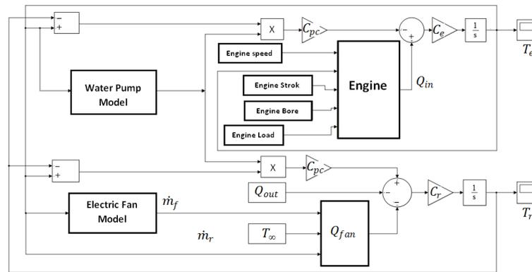
Figure 2. Electrically controlled engine cooling system model in MATLAB/SIMULINK
