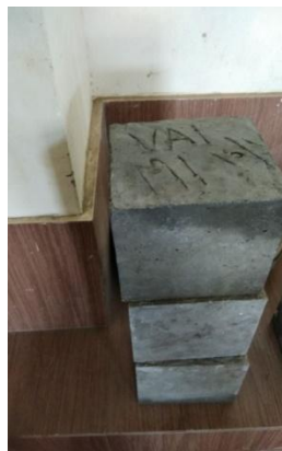
Fig.6 Eroded cubes after immersion
