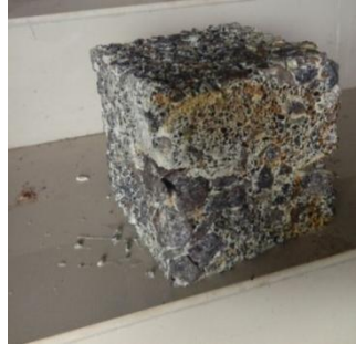
Fig 5. Eroded cube after immersion
