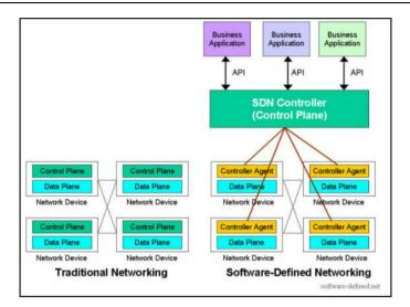
The traditional and yet existing system consists of networking elements that posses both the control and the data plane in every element that is installed in the network. This puts a slight disadvantage as setting up a new element would require making changes in control plane of almost every element that exists in the network. This leads to decrease in optimality goal of the network.
