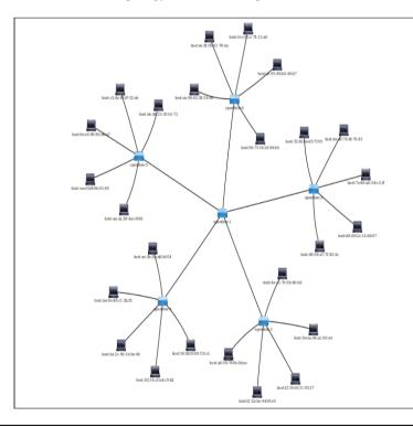
This Topology has the SDN controller at the center. Each switch including the controller has 5 connections. So in all it has 1 controller 5 switches and 25 nodes.
