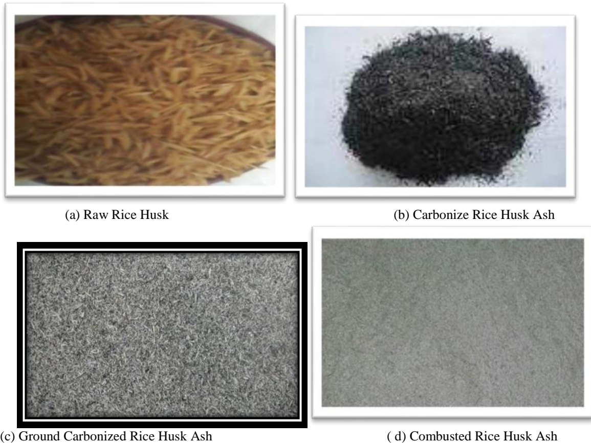
Figure1: Preparation of Rice Husk Ash
