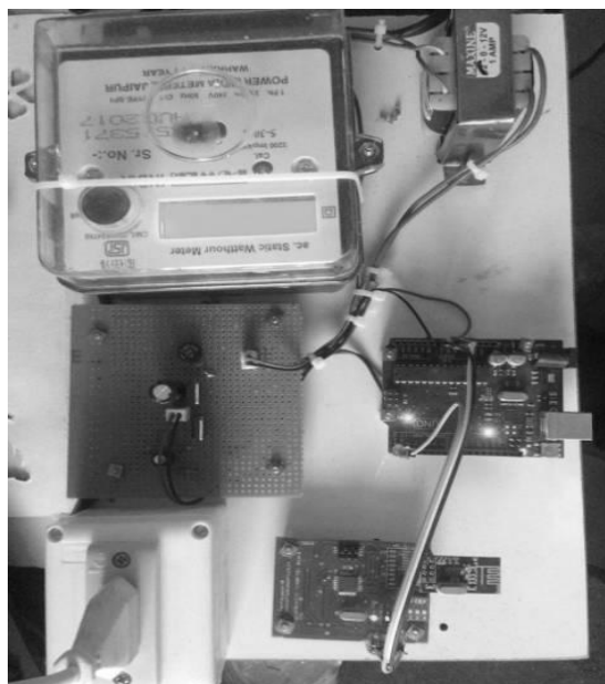
Figure 3. EMS Transmitter End
