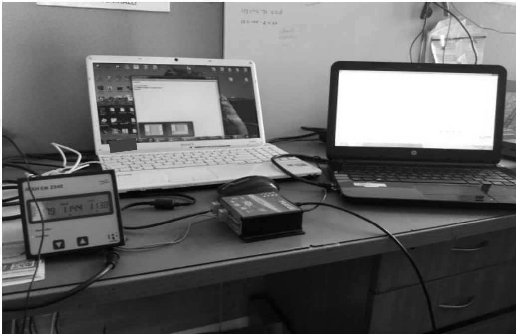
Figure10. Smart Meter interfaced with Communication Gateway
