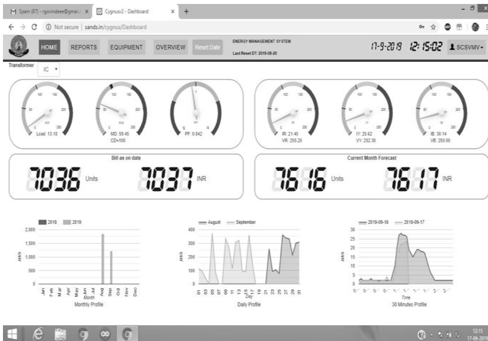
Figure 12. Electrical Parameters Obtained by the Cloud Computing based Energy Monitoring System
