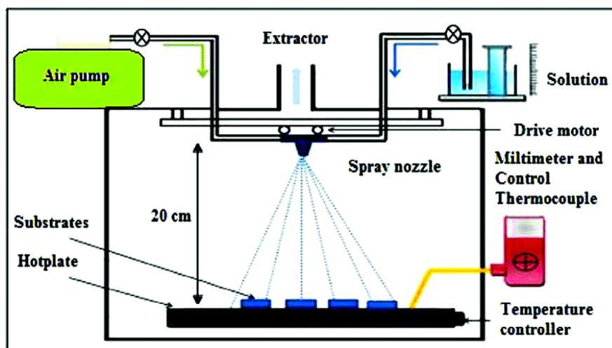
**Fig. 1 Schematic of spray deposition**
