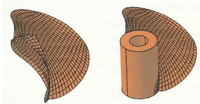
Blade model in CATIA V5 R17 software (left), model to hub surface
