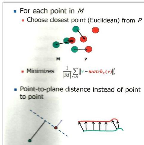
The point to point ICP method uses each 3D point within the scan data to maximize the alignment accuracy. The multiple scans are first roughly aligned via reference spheres and then the ICP algorithm is employed to align each scan using overlapping geometry to minimize global distortion.
