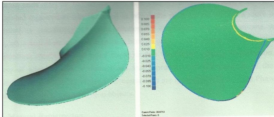
**Cleaned unwanted data (left) deviation of point cloud data to reduce noise operation (right) from actual scanned data**
