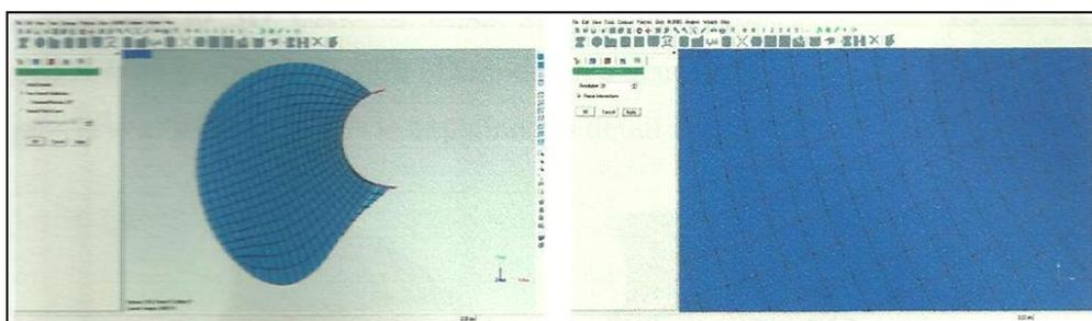
Patch construction (left) and grids construction to patch boundary (right)
