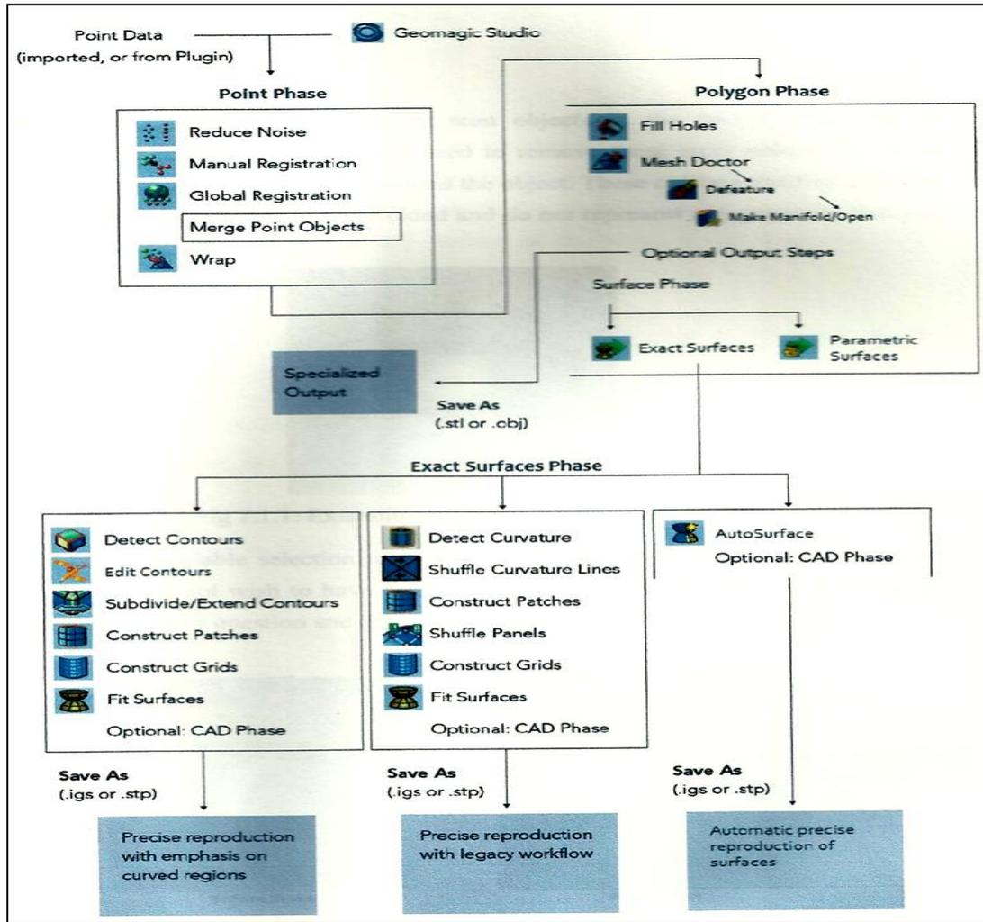
**Work flow chart in Geomagic Studio for construction of surface from scanned point cloud data**
