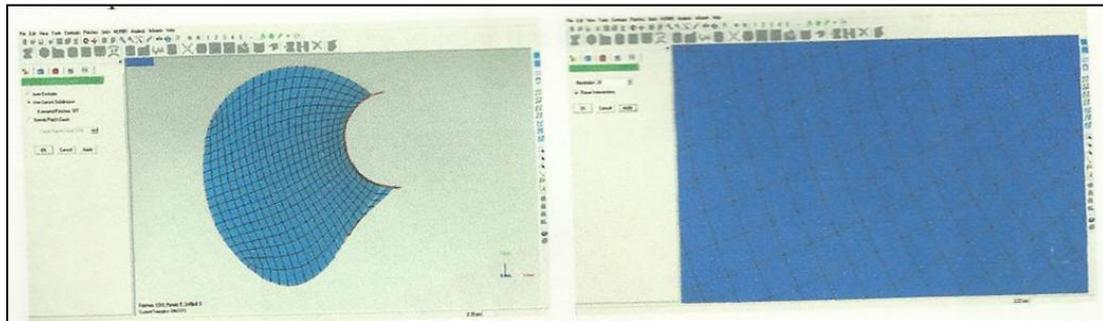
**Rectangular patch on polygon model (left) and grids construction (right)**
