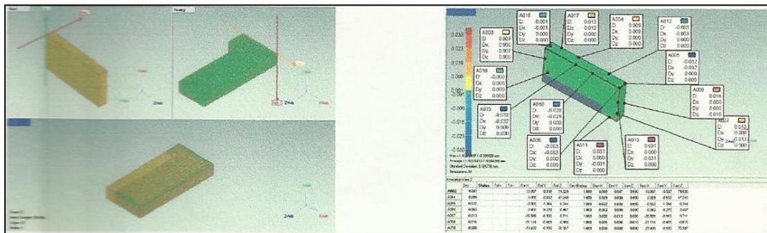
Alignment and 3D comparison of surface model with nominal CAD data
