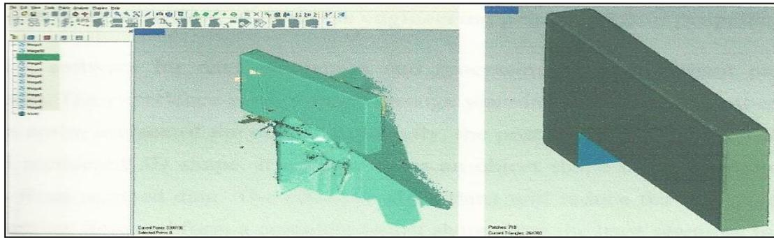
Surface conversion gauge block (CAD) from point cloud data
