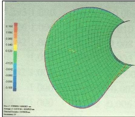
In order to evaluate the developed method, the recovered shape was compared with shape recovered by the 3D laser scanner (scanned points data). The laser scanner is considered as an accurate tool to get real values of the objects. X, Y, Z are width, height and depth of the objects respectively. The error was calculated by the difference between values obtained by the scanner and the values recovered by the proposed method.
