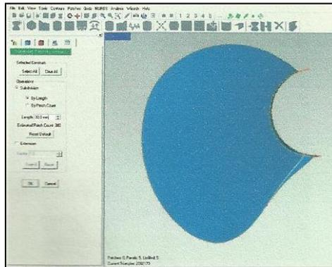
Contour lines extraction and sub division of contour lines
