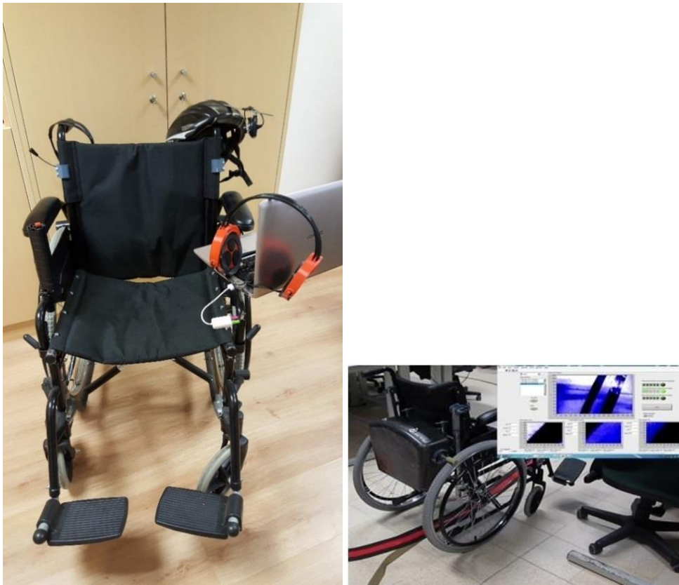
Figure 2: The low cost autonomous IPL/IT wheelchair system, with voice command, eye movement detection, GPS, colored line follower, and sound produced by scanned objects
