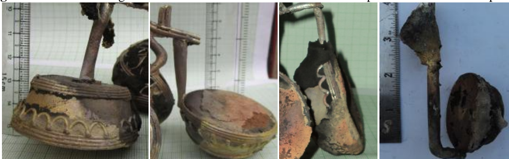
Figure 6: Pictorial View of (a): Type-I: Central Axial Top Gating system, (b): Type-II: Peripheral Axial Top Gating system, (c): Type-III: Peripheral Radial Top Gating system, (d): Type-IV: Peripheral Radial Bottom Gating system of Cosmetics Case
