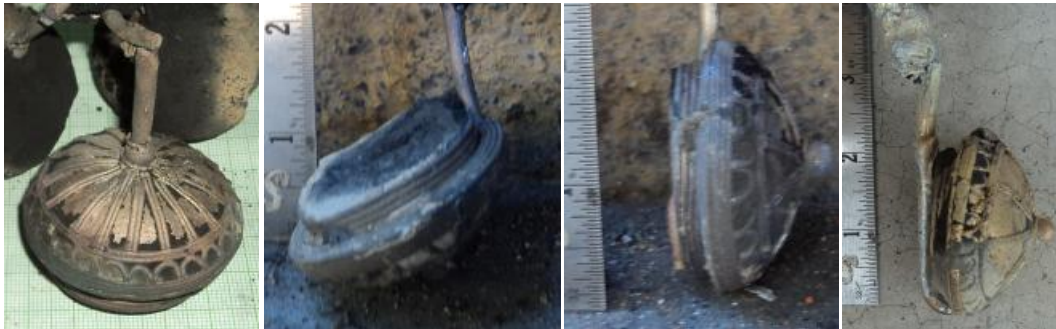
Figure 7: Pictorial View of (a): Type-I: Central Axial Top Gating system, (b): Type-II: Peripheral Axial Top Gating system, (c): Type-III: Peripheral Radial Top Gating system, (d): Type-IV: Peripheral Radial Bottom Gating system of Cosmetics Case
