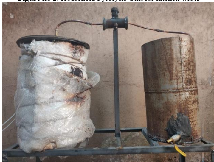
Figure no 1: Household Pyrolysis Unit for kitchen waste
