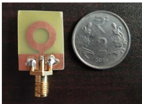
Fig. 10 Fabricated prototype of slotted CPW feed UWB Antenna
