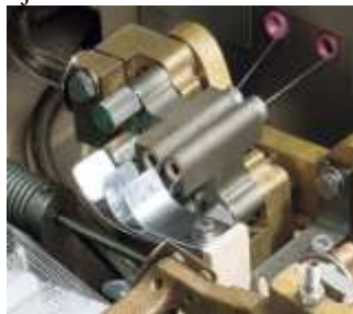
Fig. 3 Gripper Mechanism of WaterJet Looms
