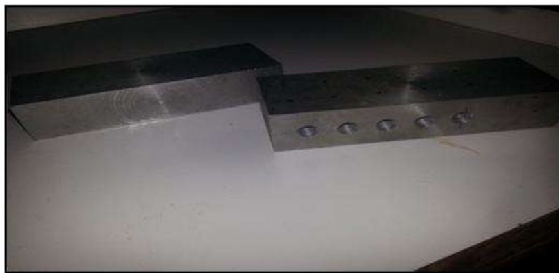
Fig.1: Solid and perforated fins
