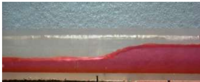
Fig.2. Hydraulic jump in a horizontal test-section without air flow ( Q_w = 2.0 \times 10^{-4} \text{ m}^3/\text{s} , Q_a = 0.0 ), ( h_1 = 10 \text{ mm} , h_2 = 30 \text{ mm} )
