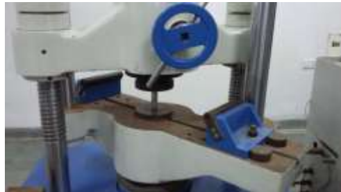
Sample put on UTM machine
