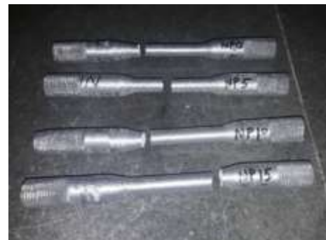
Sample break after tensile test
