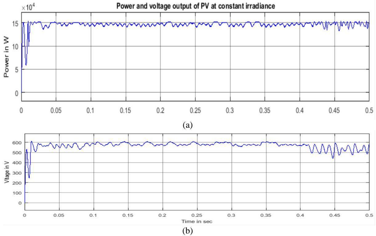
Figure 5 (a) Output power and (b) voltage of PV panel
