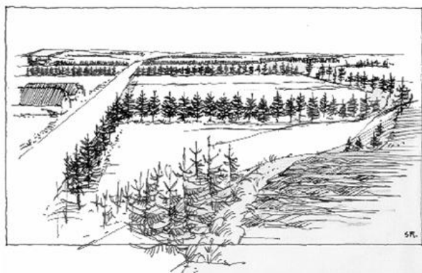
Figure 6. The terrain as the roughness class of 3: urban areas, forests, farmland with many separate wind flows. The length of roughness z_0 = 0.40 m.
