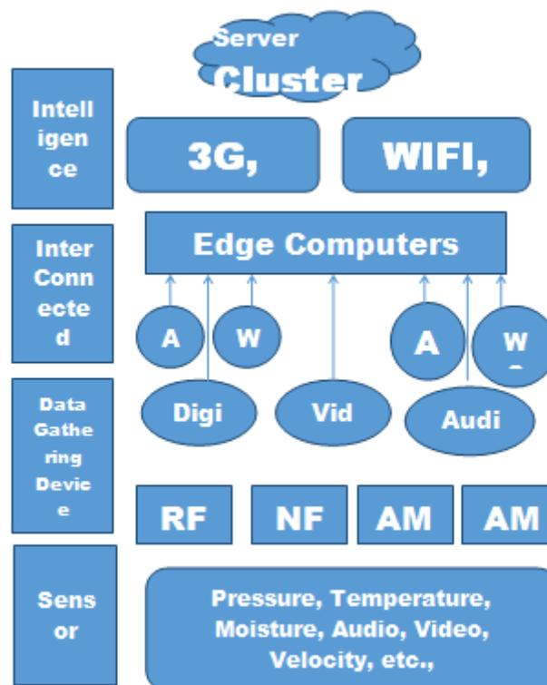
**Figure 3.1** Architecture of IoT
