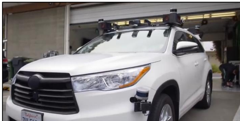
Figure 12: Add-On Autonomous Vehicle Robot
